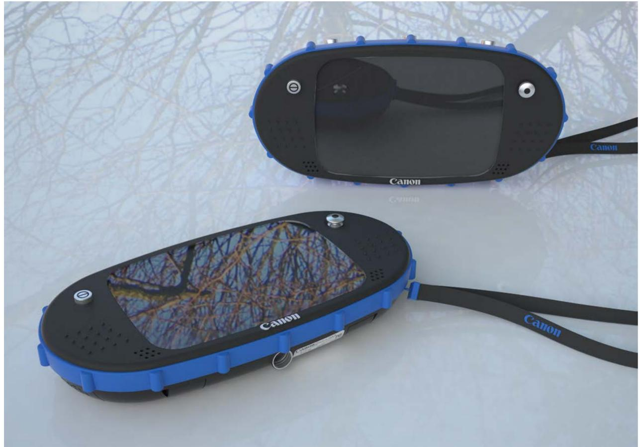
CAD RENDERINGS OF A DIGITAL CAMERA DESIGNED TO BE AS EASY TO USE AS POSSIBLE, THE CASING IS MADE OF RUBBER FOR BETTER DURABILITY.
